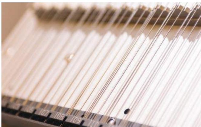
Straight length wires before placement in the wire-bending machine
